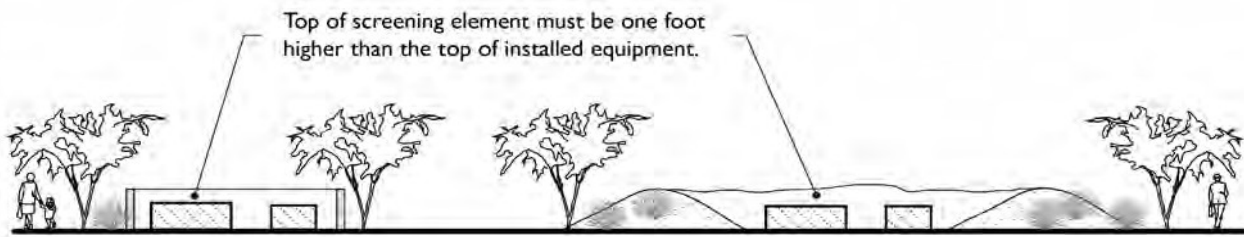
FIGURE 9-400.070-2: SCREENING OF GROUND MOUNTED EQUIPMENT
