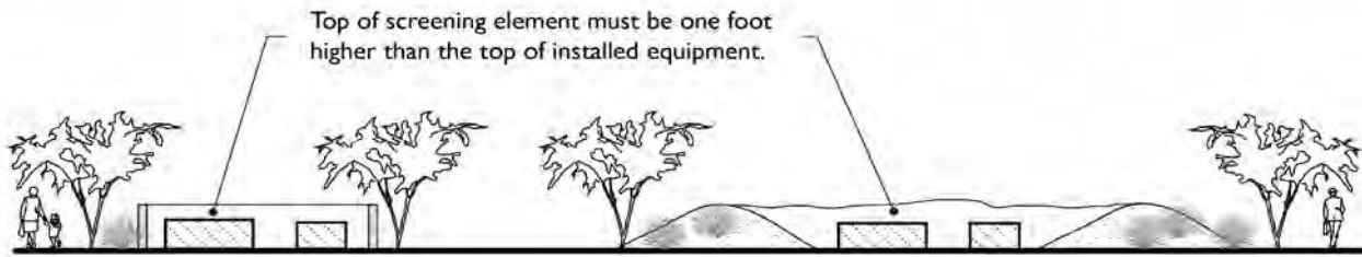
FIGURE 9-400.070-2: SCREENING OF GROUND MOUNTED EQUIPMENT
