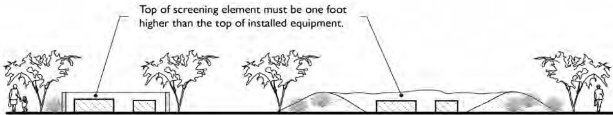
FIGURE 9-400.070-2: SCREENING OF GROUND MOUNTED EQUIPMENT
