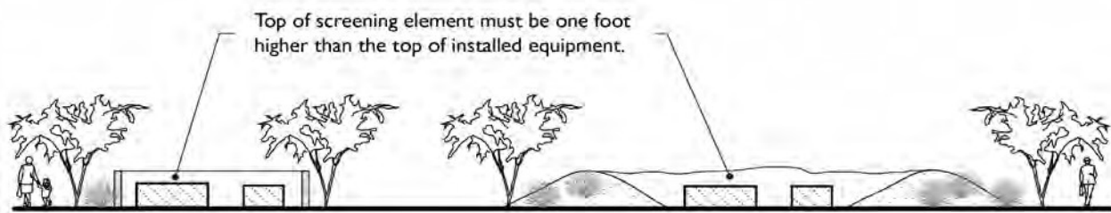
FIGURE 9-400.070-2: SCREENING OF GROUND MOUNTED EQUIPMENT
