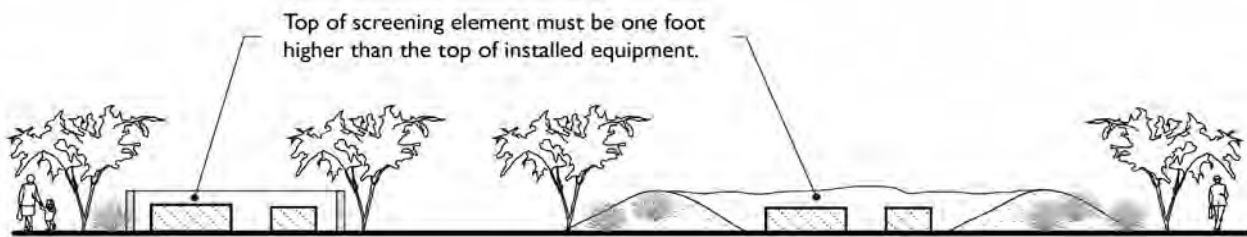
FIGURE 9-400.070-2: SCREENING OF GROUND MOUNTED EQUIPMENT
